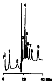
Fig. 3. Chromatogram of standard ions using lithium p -hydroxybenzoate after the position of the anion and cation columns is reversed. Other chromatographic conditions are shown in Fig. 2. Peaks: 1 = sodium; 2 = potassium; 3 = fluoride; 4 = chloride; 5 = nitrite; 6 = bromide; 7 = nitrate; 8 = phosphate; 9 = sulfate.
